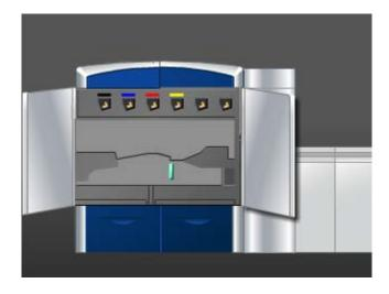
2. Lift lever **2e** to remove jammed paper.
