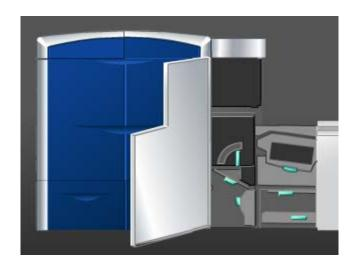
2. Grasp handle **5** and rotate it in the direction of the arrow, and slowly pull out the fuser until it stops.
