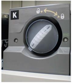
4. Remove and dispose of the empty cartridge according to local regulations.
