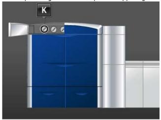
3. Rotate the cartridge to the unlock position, as shown in the following illustration.
