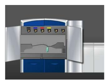
2. Use a damp, water-moistened (not wet), lint-free cloth to clean the paper path only in the green lever jam clearance areas as shown in the illustration.
