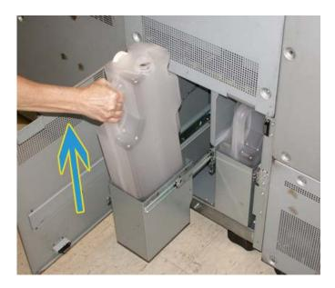
4. Remove the cap from the cap holder on the side of the full bottle, and press the cap securely into the open hole on the top of the full bottle.
