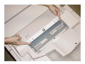
3. Load the paper/tabs, aligning it to the front side of the tray.
