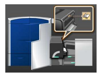
4. Grasp the handles on the fuser web assembly and pull it up and out to remove the assembly.
