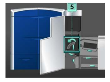
3. Push down on the lever; the fuser exit area opens.
