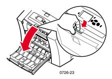
2. Pull out the maintenance drawer (labeled A), if it is not locked.
