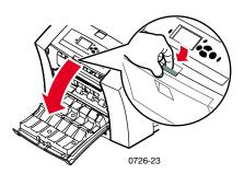
2. Remove the Maintenance Drawer (labeled A) and place it in a plastic bag for storage.
