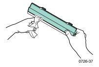
5. Make sure the thin, white dust shield is lying on top of the metal shaft. Then, reinstall the Rapid Release Guide, pressing down on the green tabs to snap the guide into place.
