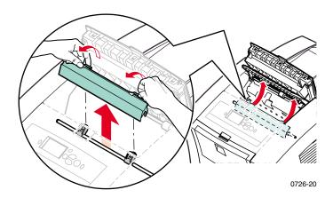
**4.** Gently clean the plastic Rapid Release Guide by wiping it with a pre-soaked alcohol cloth (using 90 percent isopropyl alcohol).
