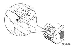
4. If necessary, adjust the guide on the right side of the slot for Letter-size (and Legal-size) or A4-size paper.
