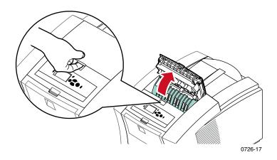
2. Using both hands, remove the jammed paper. If the paper is still caught inside the printer, skip to Solution 3 (Step 2).
