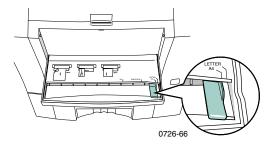
5. When the front panel displays the **Waiting for Manual Feed** prompt, insert one sheet or envelope into the manual feed slot until the printer pulls it in.
