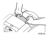
2. Remove the entire sheet of paper; any pieces left in the printer may cause more jams.
