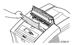
5. Make sure the thin, white dust shield is lying on top of the metal shaft. Then, reinstall the Rapid Release Guide, pressing down on the green tabs to snap the guide into place.
