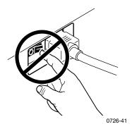
Do not move the printer while printing. Refer to page 69 for instructions for moving the printer.
