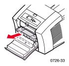
3. Use a lint-free cloth to clean the top and upper edges of the flexible plastic wiper blade located on the top of the maintenance drawer between the roller and waste tray.
