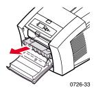
3. To clean the rollers in rows 1, 2, and 3, use a pre-soaked alcohol cloth (using 90percent isopropyl alcohol). To turn the rollers in rows 1 and 3, turn the green thumbwheel.
