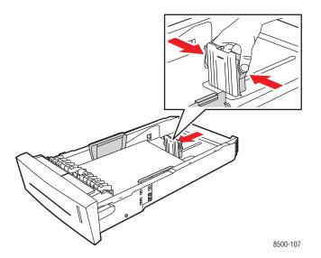
■ Width guides: Slide the width guides until the arrows on the guides point to the appropriate paper size labeled on the bottom of the tray. When properly positioned, the guides click into place.
