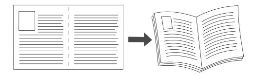
When you print booklets, you can also specify the *creep* and *gutter* in both Windows 98 and Windows Me drivers. The gutter is the horizontal distance from the fold to the page image (in points). The creep is the distance that page images are shifted inward (in 10ths of a point); this compensates for the thickness of the folded paper, which otherwise would cause the inner page images to shift slightly outward.
