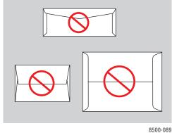
**Caution:** Never use envelopes with windows or metal clasps; they can damage the printer. Damage caused by using unsupported envelopes is not covered under the Xerox warranty, service agreement, or Total Satisfaction Guarantee. The Total Satisfaction Guarantee is available in the United States and Canada. Coverage may vary outside these areas, please contact your local representative for details.
