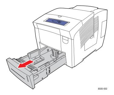
2. Insert a maximum of 400 sheets of labels into the tray with the side to be printed **faceup** and the **top** of the page toward the **front** of the tray.
