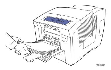
Single-sided printing: Insert the side to be printed facedown with the top of the page entering the printer first.
