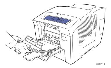
**4.** Adjust the paper guides to fit the labels loaded in the tray.
