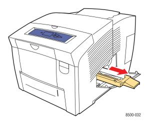
**3.** Remove the waste tray (labeled **B**) from the waste tray slot.
