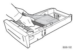
2. Insert a maximum of 40 envelopes into the tray, **flap side down** with the flap toward the **left** side of the tray.
