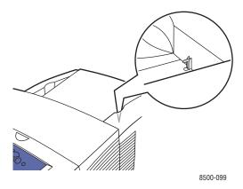
**5.** Wait for the printer to complete the cool-down period for the ink to solidify. The fan shuts down when it is cool enough to move.
