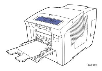
**2-sided printing**: Insert side one **faceup** with the **bottom** of the page entering the printer first.
