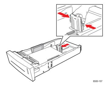
**b. Width guides**: Slide the width guides until the arrows on the guides point to the appropriate paper size labeled on the bottom of the tray. When properly positioned, the guides click into place.
