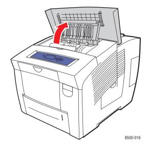
**b.** Pull the jammed paper slowly out of the printer. Confirm that any torn pieces of paper are removed.
