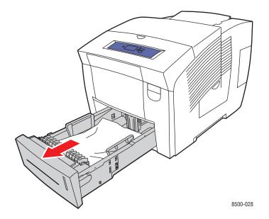
**b.** Remove any jammed paper from inside the tray slot. Confirm that any torn pieces of paper are removed.
