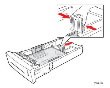
**Width guides**: Slide the width guides until the arrows on the guides point to the appropriate paper size labeled on the bottom of the tray. When properly positioned, the guides click into place.
