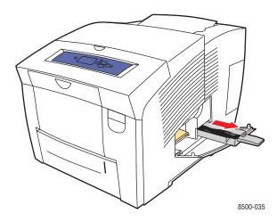
**Note:** The waste tray may be locked if the printer is in a warm-up cycle or if the ink is cooling following the **Eliminate Light Stripes** troubleshooting routine. If the tray is locked, close the door and wait 15 minutes before repeating Steps 1 and 2.
