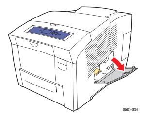
**2.** Remove the maintenance kit (labeled **A**) from the maintenance kit slot.
