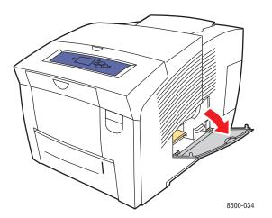
**2.** Pull the waste tray (labeled **B**) completely out of the printer.
