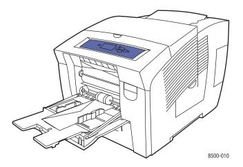
**End-flap envelopes**: Fold down the flaps before placing them in the tray. Insert the envelopes with the **flap side up** and the flap entering the printer first.
