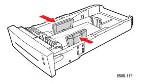
**Note:** When the paper guides are adjusted correctly, there may be a small space between the envelopes and the guides.
