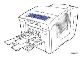
**End-flap envelopes**: Fold down the flaps before placing them in the tray. Insert the envelopes with the **flap side up** and the flap entering the printer first.
