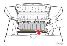
**3.** Wipe the plastic paper release blade on the lower paper guide with a pre-soaked alcohol cloth (using 90 percent isopropyl alcohol).
