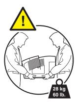
**2.** Use the original packing material and box, or a Xerox repackaging kit, to repack the printer. Do not ship the maintenance kit or waste tray with the printer.
