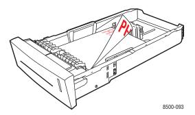
■ **Side-flap envelopes**: Insert the envelopes with the **flap side down** and the flap toward the **left** side of the tray.
