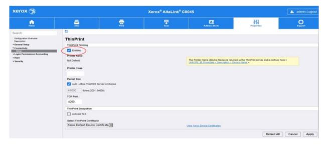
**Note:** Although a different port number can be configured, it is important not enter a port number that is already in use. ThinPrint requires a certificate to be loaded on the device when running with TLS encryption. This is located in Properties > Connectivity> ThinPrint Settings.
