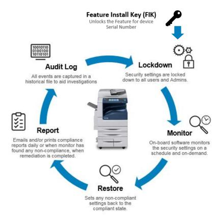
As the name implies, it "Locks down" a set of security settings on the printer, making them unchangeable to anyone including the system administrator and raises the bar on printer security. The security settings that Xerox® Lockdown Security Solution permanently controls:
