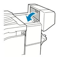
2. If the staple cartridges are not visible, grip the vertical panels at the left and right of the opening and slide them to the center.
