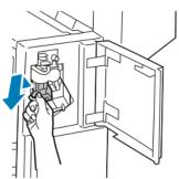
5. Pinch both sides of the staple pack and remove the staple pack from the cartridge.
