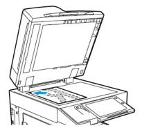
• For multiple, single, or 2-sided pages, use the duplex automatic document feeder. Remove any staples and paper clips from the pages. Insert the original documents face up in the duplex automatic document feeder, with the top of the page entering the feeder first. Adjust the paper guides so that they fit against the original documents.
