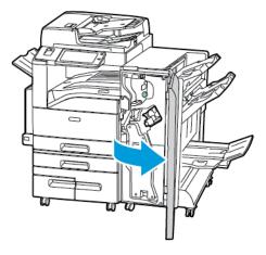
2. Grasp the booklet maker handle and pull the unit toward you until the staple cartridges appear on the top edge of the device.
