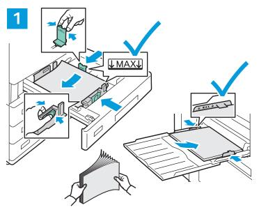
For the best results, fan the edges of the paper. Adjust the guides to fit the paper size. Do not load paper above the maximum fill line.
