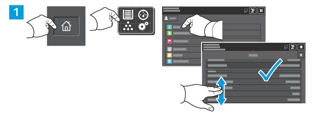
Note the printer IP address on the touch screen. If the IP Address does not appear in the upper left corner of the touch screen, press Home, touch **Device > About** then scroll to check the IP Address.
