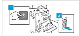
To restart the printer, on the control panel, press the **secondary power switch** (1).
