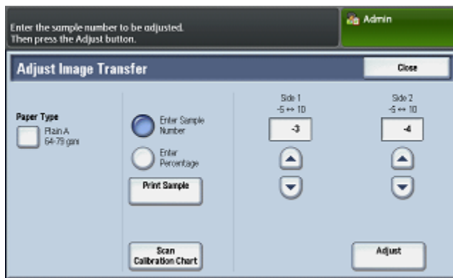
Adjust Image Transfer screen showing machine-chosen values for Side 1 and Side 2 after calibration
