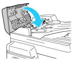
4. If the original is not visible when the document feeder top cover is opened, lift the document cover and remove the original.
