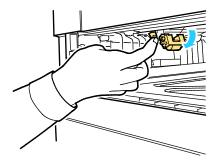
e. Grasp and pull the pick roller assembly straight down to remove it from the printer.
