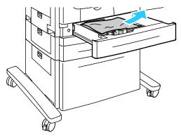
5. Push the tray completely back into the printer.
