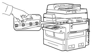
2. Open and close the top left side door so that the exit roller turns against the cloth.
