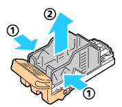
4. Insert the front side of the new staple case into the staple cartridge (1), then push the rear side into the cartridge (2).
