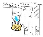
3. Pinch both sides of the staple case (1) and remove the staple case from the cartridge (2).
