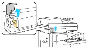
2. Grip the staple cartridge by the orange handle and remove it by pulling it to the left.
