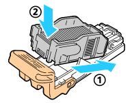
5. Grip the new staple cartridge by the orange handle and insert the cartridge into the stapler until it clicks.
