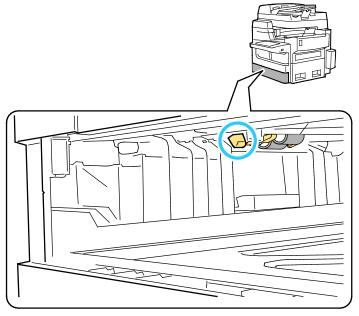
d. Raise the release lever, which allows the roller assembly to swing down.
