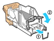
5. Grip the staple cartridge by the orange handle and insert it into the stapler assembly. Push it in until it clicks.
