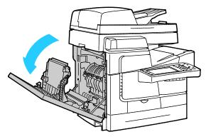
2. Lift the exit guide handle and hold it up while completing the next step.
