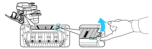
3. To rotate the paper guide to its raised position, lift the green handle.
