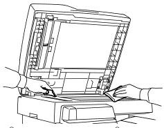
2. Use a lint-free cloth and Xerox<sup>®</sup> Cleaning Fluid or Xerox<sup>®</sup> Film Remover to clean the underside of the document cover and the document feeder.
