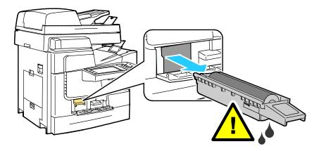
3. Remove the waste tray from the printer.
