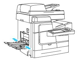
Load end flap envelopes with the flaps closed, flaps up, and flaps on the leading edge, going into the printer.
