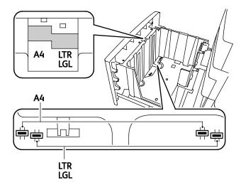
Note: To allow the plate to drop into place when aligning the front guide plate, the middle tab must be aligned properly.
