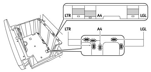
c. Lower the tabs at the bottom of the guide into the slots in the bottom of the tray. Click the top tab into the slot at the top of the tray to lock it.
