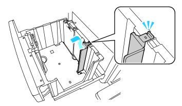
Note: Do not force the guide into place. If properly aligned, the top tab locks into the slot with light pressure.
