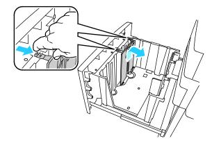
b. Align the tabs at the top and bottom of the guide with the corresponding slots at the top and in the bottom of the tray.
