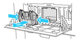
c. Inside the printer, locate the orange release lever to the left of the gray pick roller assembly.
