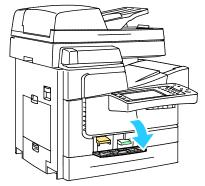
2. Remove the cleaning unit and place it in a plastic bag for storage.
