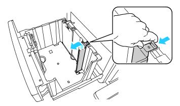
b. Align the tabs at the top and bottom of the guide with the corresponding slots at the top and in the bottom of the tray.
