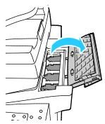
3. Place the solid ink into the opening of the appropriate ink loading bin. Do not force the solid ink into the bin. Each color is shaped uniquely to fit into the correct bin.
