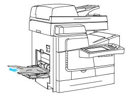
2. If you did not find jammed paper, push up the latch on the left side of the printer to open the top left side door.
