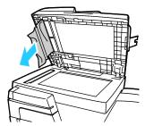
5. If the original is not wrinkled or torn, reload it into the document feeder, then follow the instructions on the touch screen.
