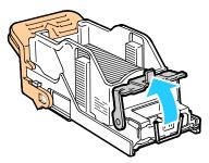
4. Remove the jammed staples (1), then push the clamp in the direction shown until it snaps into the locked position (2).
