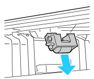
To clean the pick roller, lay a strip of clear packing tape on a table, sticky side up. Run the pick roller assembly along the length of the tape.
