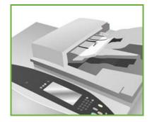
2. Lift up the Document Feeder. Place the document face down onto the Document Glass and register it to the arrow at the top right rear corner. Close the Document Feeder.
