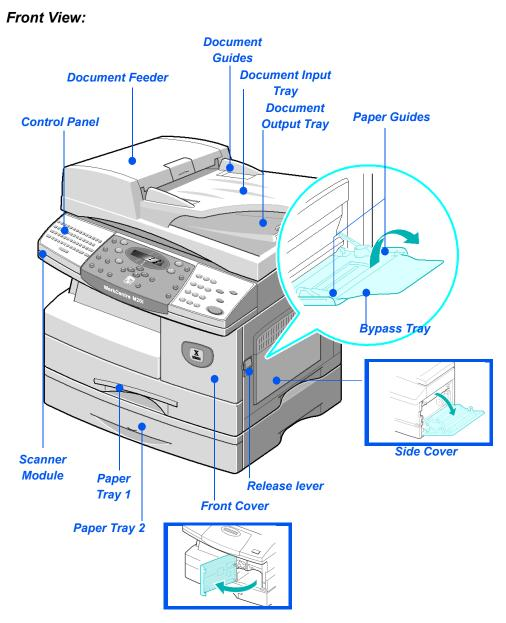
**NOTE:** The components on each model vary, this picture represents the WorkCentre M20i with the optional Paper Tray 2.
