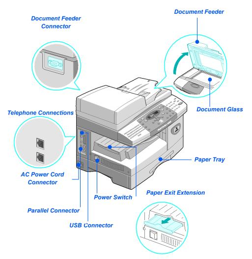
**NOTE:** The components on each model vary, this picture represents the WorkCentre M20i, standard configuration.
