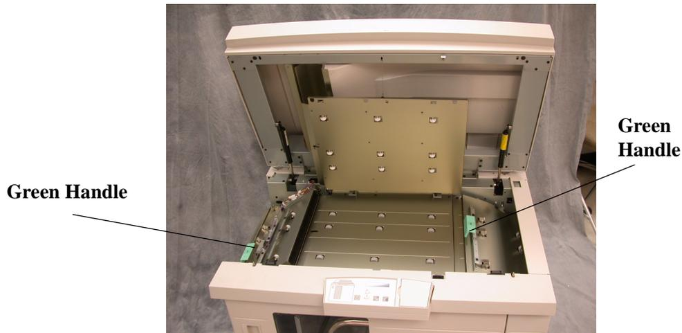
**Figure 40. EHCS Bypass Jam Clearance Areas**
