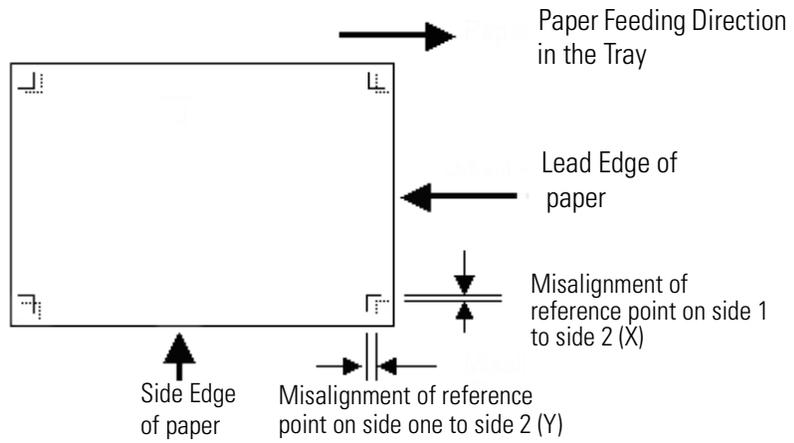
Figure 39. Measuring Misregistration
