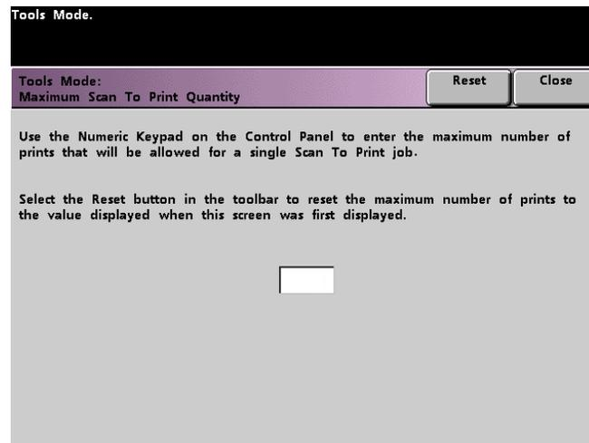
*Figure 57. Maximum Scan to Print Quantity screen*
