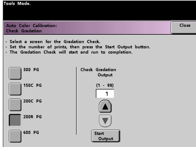
Figure 13. Check Gradation screen
