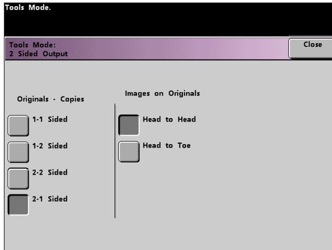
Figure 79. 2 Sided Output screen with 2-1 Sided Output selected
