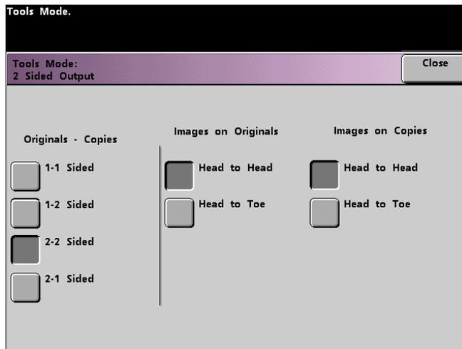
Figure 78. 2 Sided Output screen with 2-2 Sided Output selected
