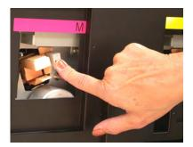
4. Verify that both the corotron assembly and the cleaning wand are seated properly.
