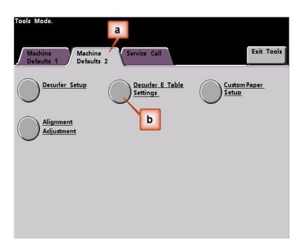
Curl remains after you have tried the System Default and the Decurler Paper Type A-D Settings. See "Decurler Paper Type A - D Settings" on page 3. As a result, you need to program the Decurler to use downward pressure (or the lower roller) to remove the downward (bridged) curl.
