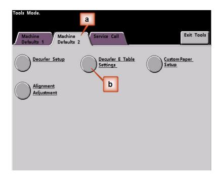
Curl remains after you have tried the System Default and the Decurler Paper Type A-D Settings. See "Decurler Paper Type A - D Settings" on page 3. As a result, you need to program the Decurler to use upward pressure (or the upper roller) to remove the upward (cupped) curl.
