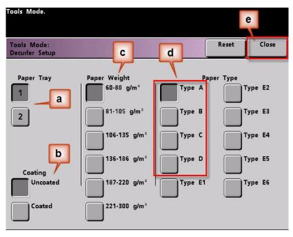
**NOTE:** Touch the **Reset** button on the Decurler Setup screen to return to the settings established when you first accessed the screen. As an example, if the system automatically selected Type B and you changed it to Type C, the system will return the setting to Type B.
