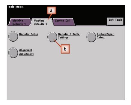
4. Curl remains after you have tried the System Default and the Decurler Paper Type A-D Settings. See "Decurler Paper Type A - D Settings" on page 3. As a result, you need to program the Decurler to use upward pressure (or the upper roller) to remove the upward (cupped) curl.
