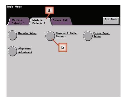
4. Curl remains after you have tried the System Default and the Decurler Paper Type A-D Settings. See "Decurler Paper Type A - D Settings" on page 3. As a result, you need to program the Decurler to use downward pressure (or the lower roller) to remove the downward (bridged) curl.
