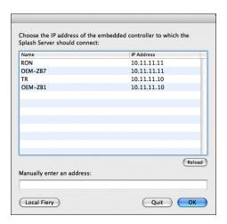
**NOTE:** For Direct Connect, you are already connected to the Fiery and do not need to select the Fiery. If the Direct Connect configuration is incorrect, the following window may appear.
