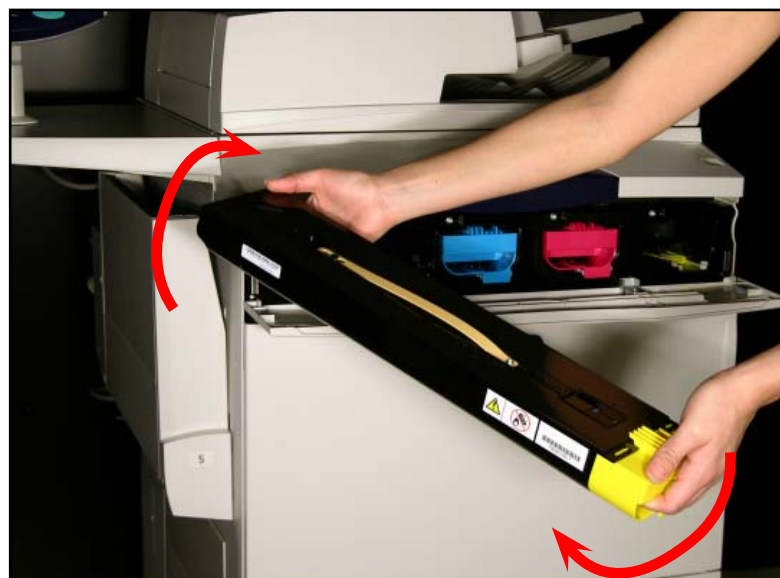
Fig. 4 Lightly shake the “new” toner cartridge three or four times up and down and to the left and right.
