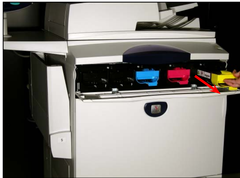
Fig. 3 Pull the toner cartridge indicated in the message on the display out.
