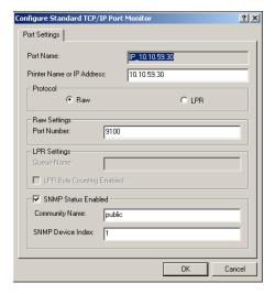
12 If LPD printing is enabled on the Fiery EXP50, select LPR in the Protocol area and LPR Byte Counting Enabled in the LPR Settings area.
