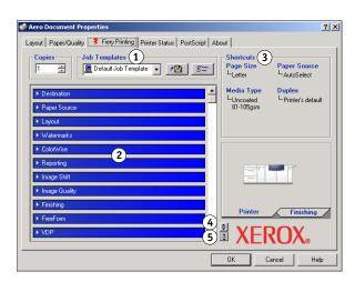
The Fiery Printing tab serves as the control center for all frequently used printing functions.
