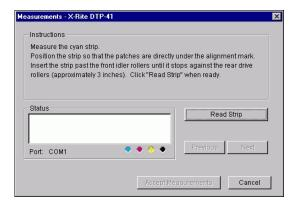
Align the page in the measurement page slot of the DTP41 so that the appropriate color column is centered below the alignment mark. Insert the page about three inches, past the front idler rollers, until it rests against the rear drive rollers and you feel resistance.
