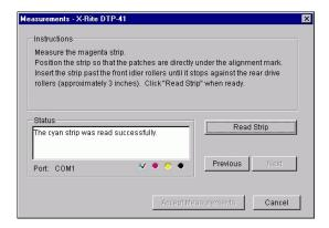
A check mark appears on the circle of the color just read, and the Status field indicates the color was measured successfully.
