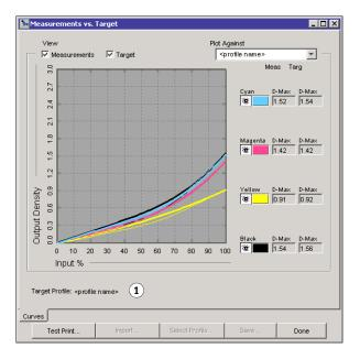
When more than one profile uses the same target, an additional menu called Plot Against appears in the upper-right corner of the dialog box. It lists all output profiles that use that same calibration set. Selecting an output profile from this menu displays the target curves associated with that profile. If each output profile contains a unique calibration target, the curves displayed also change when you switch profiles.
