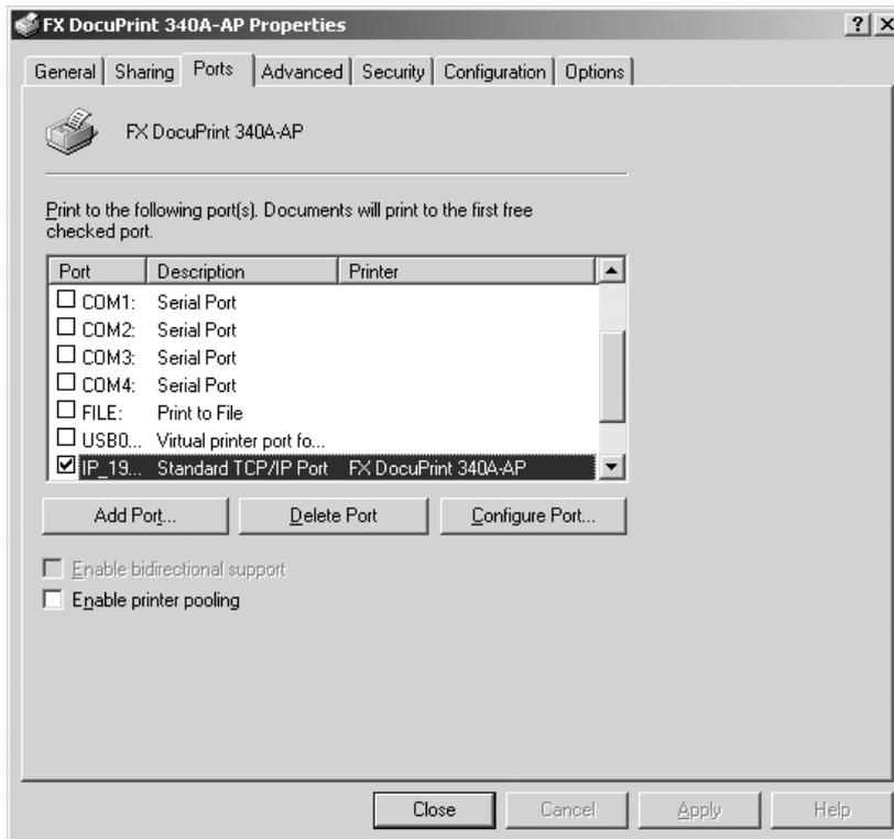
**4** Select **Raw** for Protocol. Make sure that the displayed port number is the same as the number specified at the printer. Click **OK**, and then **Apply** on the dialog box displayed to save your setting.
