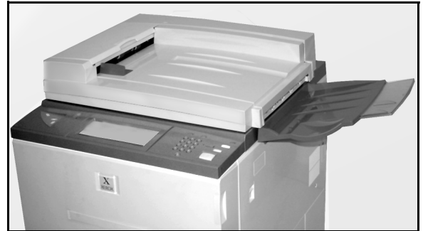
Figur 12: DADF (Duplex Automatic Document Feeder)
