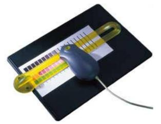
If the Spectrocam was not previously calibrated, a prompt directs you to measure/remeasure the white reference. Place the measurement device on the white target reference and touch the green sensor. After remeasuring the white reference, reposition the measurement device on the first patch on the upper
