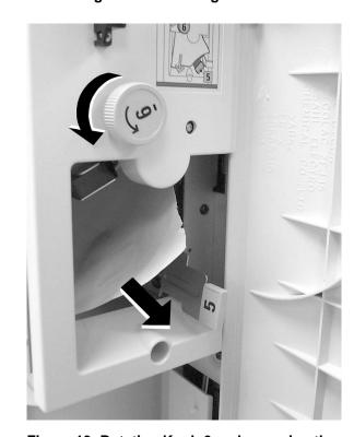
Figure 13: Rotating Knob 6 and removing the jammed paper
