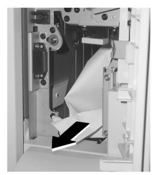
Figure 17: Removing paper from Area 8
