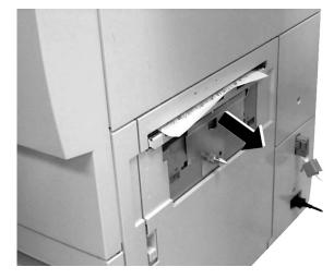
Figure 10: Removing paper from the Interface Area
