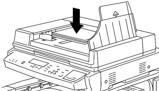
3. Gently push the originals into the Document Feeder, as shown below, until the Document Feeder light illuminates.
