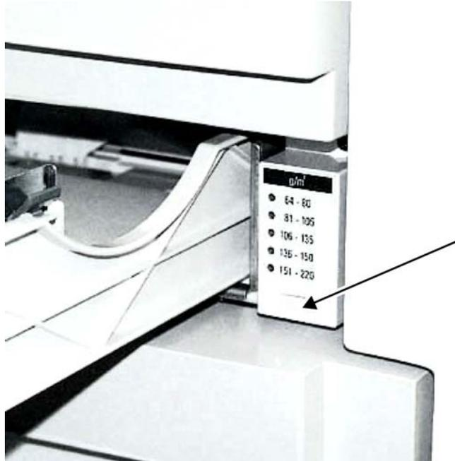
**Figure 1-3. Paper trays 1 and 2 weight indicator on the frame**
