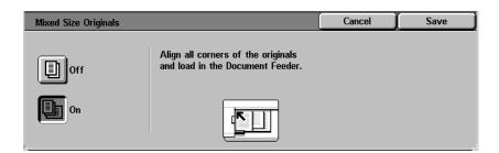
This feature automatically determines the correct paper size when scanning different size documents. The correct paper size will be determined based on the original size and the selected reduction/ enlargement.
