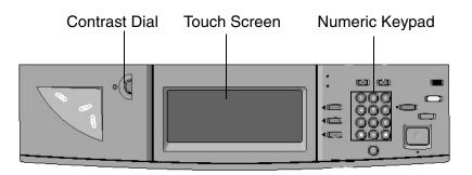
The Control Panel is used to program individual jobs.
