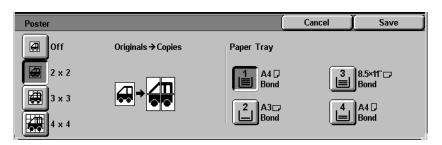
This feature allows you to create a poster size reproduction of the original document by creating multiple images that can be trimmed and joined together after. There will be a 10mm image overlap on the copies to allow for the trimming and joining required to assemble the copies into a poster.
