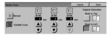
The Border Erase feature enables you to eliminate unwanted marks near the edges of the original from the output copy. The range for Border Erase is 0 through 50 mm (0.0 to 2.0 inches) in 1mm (0.1 inch) increments.
