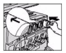
8 Rotate the cartridge clockwise until the arrow on the cartridge is aligned with the arrow and lock position on the printer/copier.
