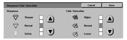
The Sharpness feature allows you to adjust the amount of edge definition on the copies. The Color Saturation feature allows you to adjust the overall richness of color on the copy. There are five levels of adjustment for each feature.
