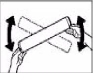
With the arrow on the cartridge facing upward, slide the cartridge into the printer/copier.
