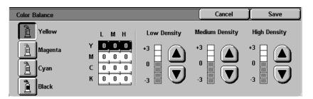
The Color Balance feature allows you to adjust the balance between colors and the overall amount of color on the output copies. You can adjust the levels of all four process colors (Yellow, Magenta, Cyan, and Black) for their low, medium and high density ranges.
