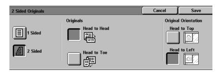
When the DADF is used for scanning, the original orientation must be set in order to specify the "Head" position of the document.
