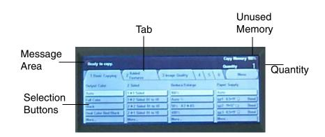
Press the buttons and tabs displayed in the Touch Screen to select features or respond to on screen instructions. The selected buttons are highlighted to indicate activation. Buttons that do not have three-dimensional shadows are not active, and cannot be selected.
