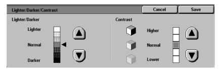
The Lighter/Darker feature enables you to adjust the overall lightness or darkness of the output copy. Contrast allows you to adjust the clearness of the image. If you increase the Contrast, the copy appears sharp & vivid and is composed of mainly high and low density elements. If you decrease the Contrast, the copy is softer and renders more uniformly using mid-tones.
