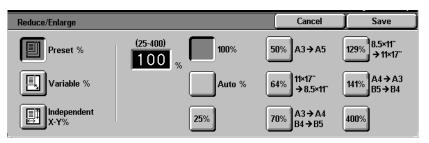
The Reduce/Enlarge feature allows you to copy the image at different magnifications. Copies may be reduced to 25% or enlarged to 400%, in 1% increments.
