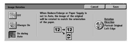
This feature allows the machine to automatically rotate the image so that the orientation of the document matches the output paper.
