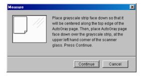
Follow the directions in the dialog box for placing the Kodak Gray Scale strip and the AutoGray measurement page on the copier glass, and click Continue.
