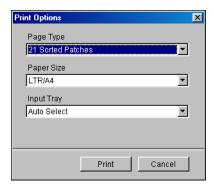
For Page Type, choose either 21 or 34 Sorted Patches, or 21 or 34 Randomized Patches. Sorted patches are printed on the page in the order of their hue and saturation levels. Randomized patches are printed on the page in random order, to help compensate for density inconsistencies on different areas of the page.
