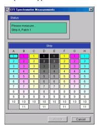
9. Place the ED-100 over the specified patch on the Measurement Page, making sure to center the sample aperture over the patch. Press Measure to take the measurement.
