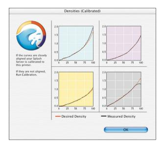
If the Measured Density levels do not match Desired Density levels, calibrate the printer again.
