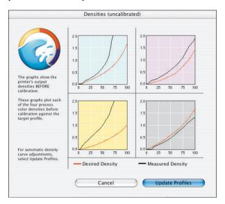
When this process finishes, ColorCal displays a graphic representation of color performance for the printer.
