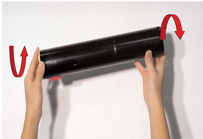
Fig. 4 Lightly shake the new toner cartridge three or four times up and down to the left and right.
