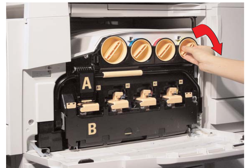
Fig. 6 Turn the toner cartridge to the right down to the key (closed).
