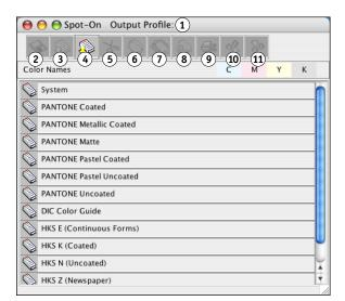
**NOTE:** When you print a job, choose the same output profile from the printer driver as the one that is selected in the Select Output Profile dialog box. Otherwise, color adjustments based on Spot-On have no effect.
