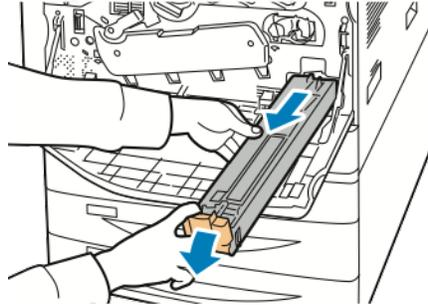
4. Place the used waste toner container in the plastic bag, then seal it firmly using the zipper.
