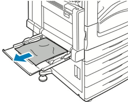
2. If the paper is torn, check inside the printer for torn pieces of paper.
