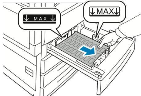
3. For short-edge feed, load labels face up with the top edge facing to the right.
