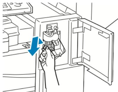
5. Remove any loose staples or other debris from inside the finisher.
