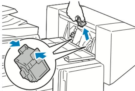
4. Hold the tabs on both sides of the new staple cartridge and insert it into the original position in the finisher.
