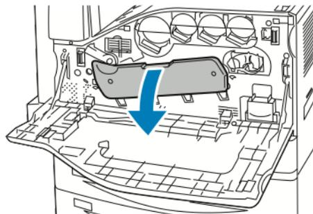
4. Grip the orange handle of the drum cartridge as shown, then pull the drum cartridge straight out of the printer. Place the used drum cartridge in the plastic bag and place in the box.
