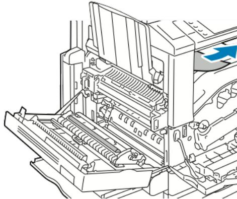
6. If paper is jammed in the fuser, pull green lever A1 to open the fuser exit gate.
