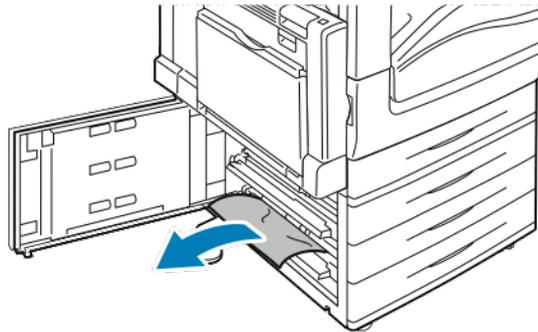
3. For paper jammed in the upper position, look inside the printer to remove it.
