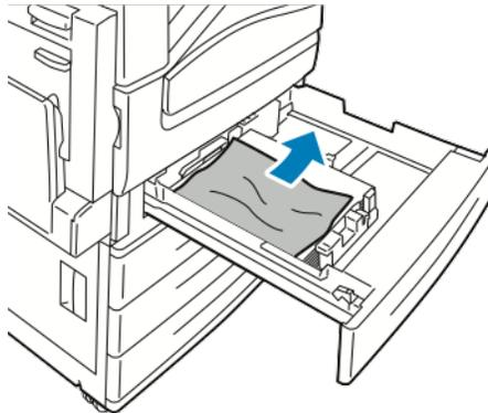
5. Reload the tray with undamaged paper, then push the tray in until it stops. Paper Settings - Tray X appears on the control panel.
