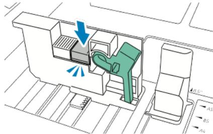
5. Load the custom-size paper in the tray. The tray guides move in increments of 1 mm (0.04 in.).
