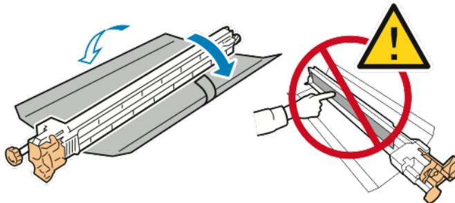
8. Support the new transfer belt cleaner with your left hand and slide it straight into the opening until it stops.
