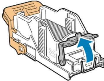
7. Remove the jammed staples (1), then push the clamp in the direction shown until it snaps into the locked position (2).
