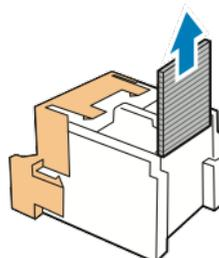
5. Hold the tabs on both sides of the new staple cartridge and insert it into the original position in the finisher.
