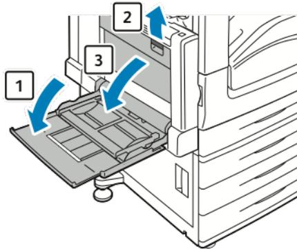
2. While lifting the release lever (2), open door B as shown (3).
