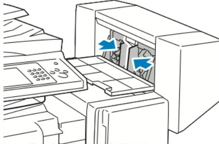
3. Hold the tabs on both sides of the staple cartridge and pull the cartridge out of the finisher.
