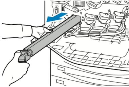
5. Remove the packing material from the end of the new drum cartridge.
