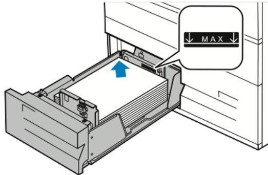
4. Adjust the guides so that they touch the edges of the stack.
