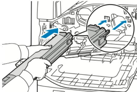
7. With the guides inserted in the slot, to remove the black paper sheet, pull it in the direction shown.
