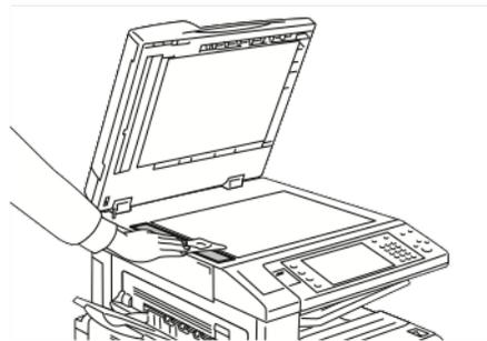
2. Use a lint-free cloth and Xerox® Cleaning Fluid to clean the underside of the document cover and the document feeder.
