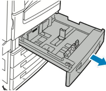
**Note:** For best results, remove any paper from the tray, pinch the guide levers, and slide the guides inward.
