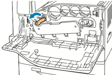
3. Pull the drum cartridge cover down until it clicks into the open position.
