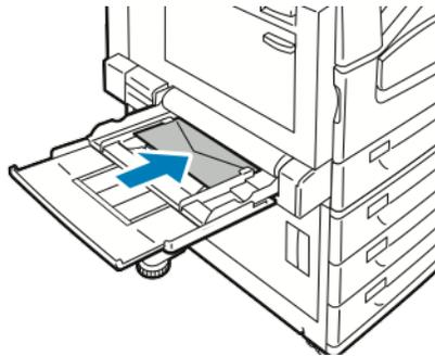
3. Center the stack, then slide the guides until they lightly touch the edges of the stack.
