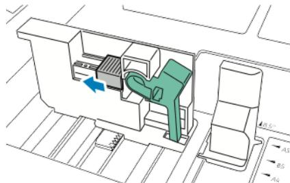
4. Replace the retainer and snap it into place.
