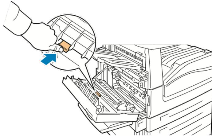
6. Lift the used transfer roller out of the printer.
