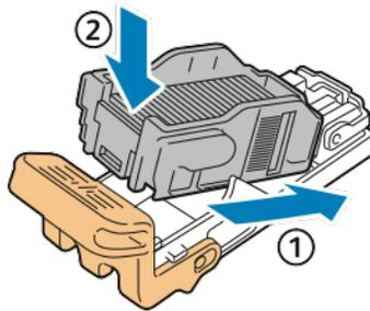
8. Grip the staple cartridge by the orange handle and insert it into the stapler until it clicks to lock in place.
