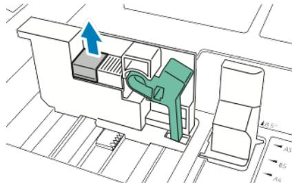
3. To engage the fine-adjustment block, pinch the levers and slide the guide lock to the left as shown.
