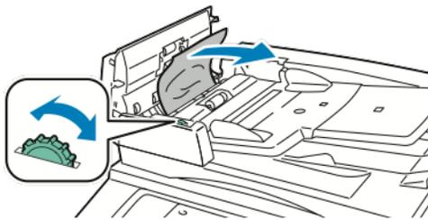
4. If the message instructs you to open the inner cover, lift the lever with the green tab to open the inner cover.
