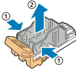
7. Insert the front side of the new staple case into the staple cartridge (1), then push the rear side into the cartridge (2).
