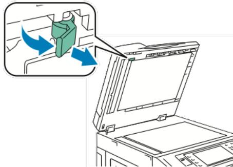
2. To separate the left end of the document cover from the lens assembly, continue to lower the lever.
