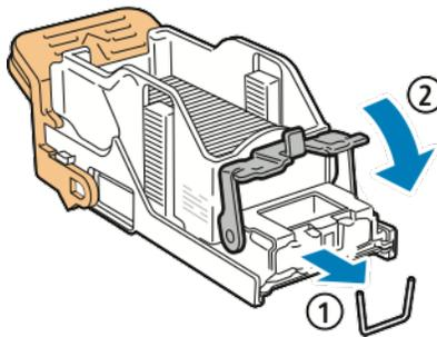
8. Grip the staple cartridge by the orange handle and insert it into the stapler until it clicks to lock in place.
