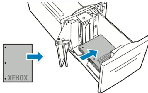
**Note:** Do not load paper above the maximum fill line. Overfilling can cause paper jams.
