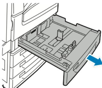
2. Ensure that the guide locks are set in the correct position for the standard or custom size paper that you are loading. For details, see [Setting the Guide Locks in the 500-Sheet Adjustable Trays](#) on page 56.
