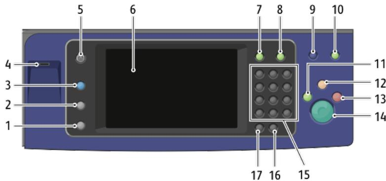
1. **Machine Status** displays the status of the printer on the touch screen.
