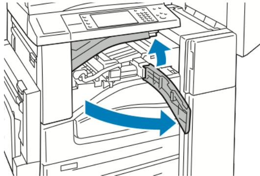
2. Pull out the hole punch waste container.
