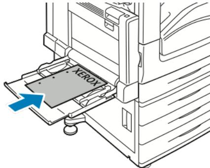
**Note:** Do not load paper above the maximum fill line. Overfilling the tray can cause the printer to jam.
