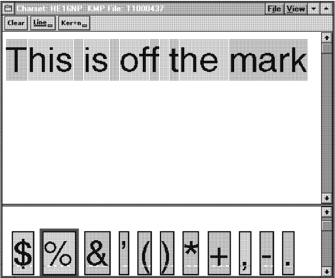
Figure 8-21. Incorrect raster-pattern box spacing example
