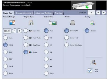
This screen includes the core copying controls for reduction/enlargement, original type, output size, destination printer and print quality.
