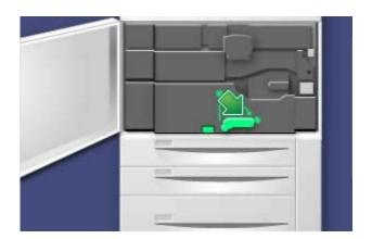
**3.** Carefully pull out the transfer module.
