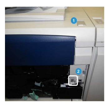
The machine has two power switches:
