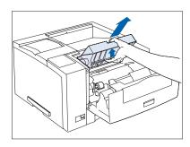
Open the front cover and remove the EP cartridge by lifting it towards the rear of the printer then pulling it up and out.
