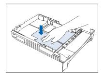
1 Press down on the bottom plate of the paper tray until it clicks into position.
