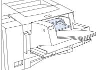
Stack the envelopes face up with the stack against the feeder's left edge.
