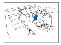
**1 4** Lift the BTR out of the printer.
