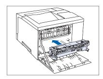
Slide the new fuser cartridge into the printer.
