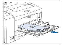
6 When feeding envelopes, slide the end of the envelope stopper over the end of the envelope stack. Refer to Figure 4.3 on page 4-13 for correct envelope orientation.
