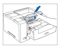
2 Remove the old EP cartridge by lifting it towards the rear of the printer then pulling it up and out.
