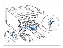
4 Remove the Duplex Module by pushing the green lock buttons on either side of it.
