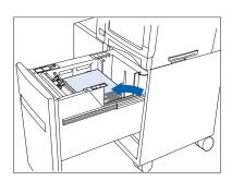
3 Load paper using the opening in the side of the drawer. Refer to Figure 4.5 on page 4-19 for correct paper orientation.
