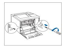
5 Remove the mounting screws from the printer as shown at left, and set them aside.
