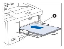
4 Insert paper along the left side of the tray, under the plastic maximum fill tab (1). Refer to Figure 4.2 on page 4-12 for correct paper orientation.
