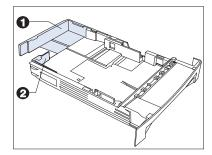
3 Slide end guide B (2) out to align it with end guide A (1).
