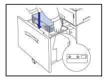
**4** Gently load the stack of paper into the tray (see illustration, below, for orientation of letterhead and drilled paper.
