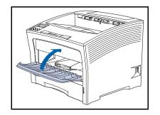
**6** the door can be closed when the media fits within the multi bypass feeder enclosure.
