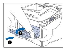
**5** If you extended the multi bypass feeder in Step 2, return it to its normal position:
