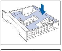
4 If the tray's metal base plate remains raised, press it down to lock it.
