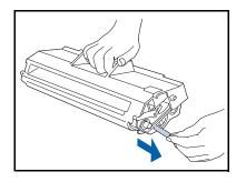
4 Place the cartridge on a flat surface, press it down with one hand and with the other grasp the end tab of the sealing tape and pull the tape straight out horizontally.
