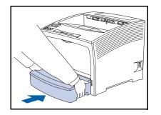
**11** Push the tray completely into the printer. Make sure it is properly seated.
