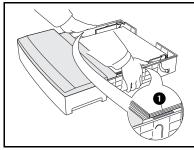
**10** Hold the tray at the green labels (1) and insert it into the printer.
