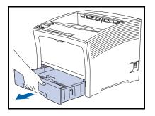
Remove the tray from the printer and place it on a flat surface.
