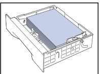
5 Align the four corners of the paper stack and insert it into the tray with the side to be printed on facing up (see illustration, below, for orientation of letterhead, drilled paper, transparencies and envelopes. Make sure the paper is placed at the center of the tray, under the retaining clips on both sides.
