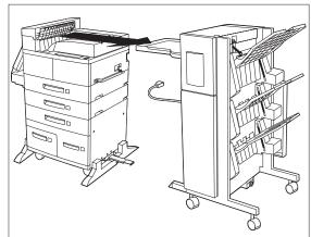
**5** Remove the finisher GFI power cord from the printer and slowly pull the finisher away from the printer.
