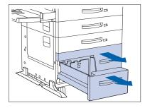
**3** Open Trays 4 and 5. Carefully remove any jammed paper. Reseat the paper in the trays.
