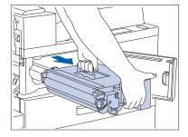
Remove the Laser Print Cartridge by lifting the amber handle and gently pulling it out.
