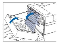
4 Close the inside cover of the Duplex Module, then close the Duplex Module.
