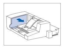
3 Slide the side guide so that it touches the edges of the envelope stack lightly.
