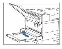
Push the paper guide slightly to touch the paper stack (to ensure contact with the paper sensor).
