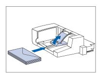
**7** Lift the envelope stopper and insert the stack with the flap-side up and the long edges leading into the printer.
