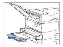
1 If necessary, pull out the extension tray to fit the length of paper to be used.
