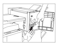
Place one hand under the cartridge. Use your other hand to release the cartridge from the Finisher by pushing down on the latch as shown.
