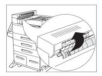
Lift the plastic roll cover under the paper transport, using the tab as indicated. Remove any paper under the roll cover. Release the roll cover when you have removed the paper.
