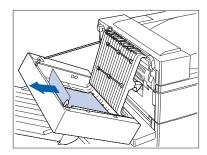
**3** Remove any jammed paper in the direction of the arrow.
