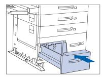
Place paper in the tray, against the left side (refer to Figure 2.3 on page 2-16 for orientation). Slide back the stop.
