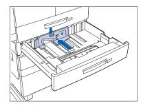
4 Press down the gray handle and slide the side guide all the way until it stops.
