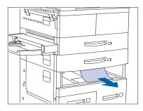
**7** Open and remove Tray 3 by lifting the tray from the front. Carefully pull out any jammed paper. Reseat the paper, then replace and close Tray 3.
