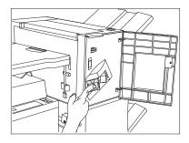
5 Slide the full Staple Cartridge into the Finisher until it snaps into place.
