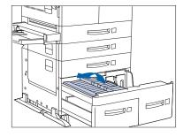
4 Lift the Tray 5 transport and carefully remove any jammed paper, then close Trays 4 and 5.
