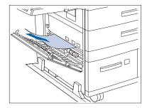
Open Door C and remove any jammed paper. Then close Door C.
