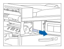
**8** Gently pull the sealing tape straight out in the direction of the arrow.
