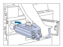
6 Hold the amber handle with one hand and gently push the Laser Print Cartridge all the way into the printer.
