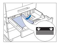
**5** Place the paper in the tray, between the guides (see Figure 2.1 on page 2-12 and Figure 2.2 on page 2-13 for orientation).
