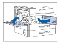
**7** Gently pull the sealing tape straight out in the direction of the arrow.
