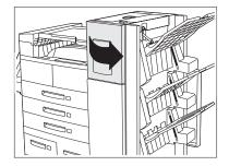
Open the access door on the side of the Finisher.
