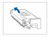
Remove the new Laser Print Cartridge from its package and pull out the protective paper sheet from the drum shutter.
