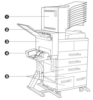
Figure 1.3 Customer replaceable components
