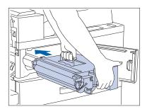
Hold the amber handle with one hand and gently push the Laser Print Cartridge all the way into the printer.
