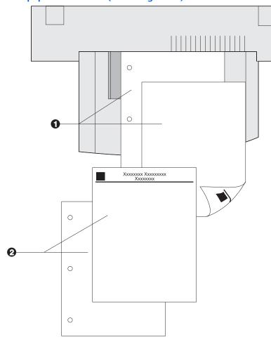
Figure 2.6 50 Sheet Bypass Feeder envelope orientation<sup>1</sup>
