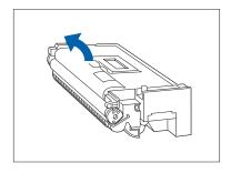
4 Remove the new Laser Print Cartridge from its package and pull out the protective paper sheet from the drum shutter.
