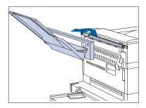
1 Remove the Face-up Bin by lifting it up and out.
