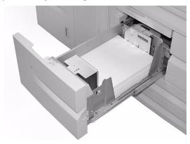
2. Load  $8.5 \times 11$  in. or A4 paper and align the edge of the paper against the left edge of the tray.
