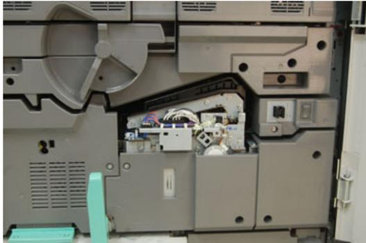
5. Locate the fuser identifier clip on the fuser assembly and, using a marker, write on the identifier the fuser width being used.
