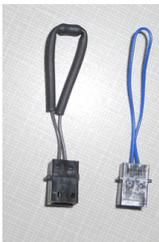
7. Attach the appropriate jumper to the exposed white connector at the front of the fuser assembly by pushing the two ends together. There is no release. To disconnect, simply pull apart.
