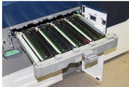
5. Remove the old drum cartridge by holding the finger rings provided at the both ends of the drum cartridge and gently lifting up.
