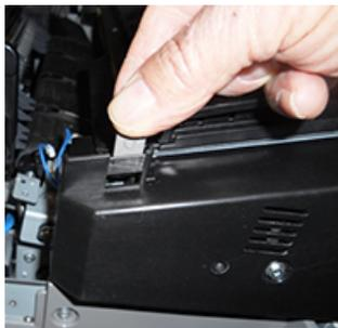
**9.** Using the provided T10 Torx driver, remove one screw and the Fuser Front Cover.
