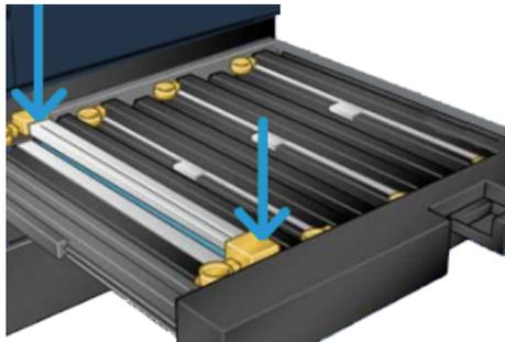
11. Immediately close the drum cartridge drawer to protect the other drums from light.
