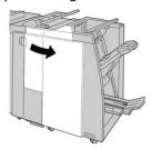
**3.** Grasp the Staple Cartridge handle located at **R1**, and pull out the staple cartridge from the finisher.
