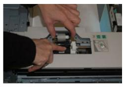
**4.** Replace the new roll by squeezing both ends of the metal shaft, and pushing down on the black tab, insert and release the roll ends into the notches.
