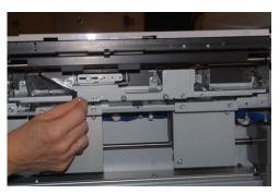
**6.** Slide the retard assembly all the way to the left so it is out of the slots. Pull the assembly out towards you until completely removed from the tray. Set aside.
