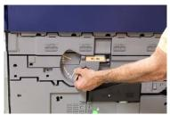
4. Open the bag containing the new drum cartridge. Place the new drum cartridge near the press.
