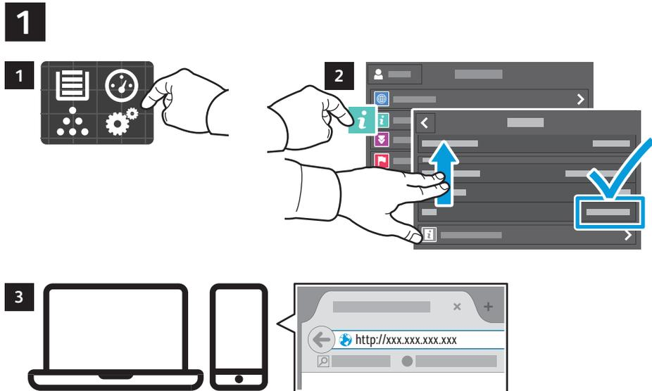
**EN** Connect to the Embedded Web Server of the printer. In a Web browser, type the IP address of the printer. The network IPv4 address is available on the control panel touch screen. Touch **Device** app > **About**, then scroll down.
