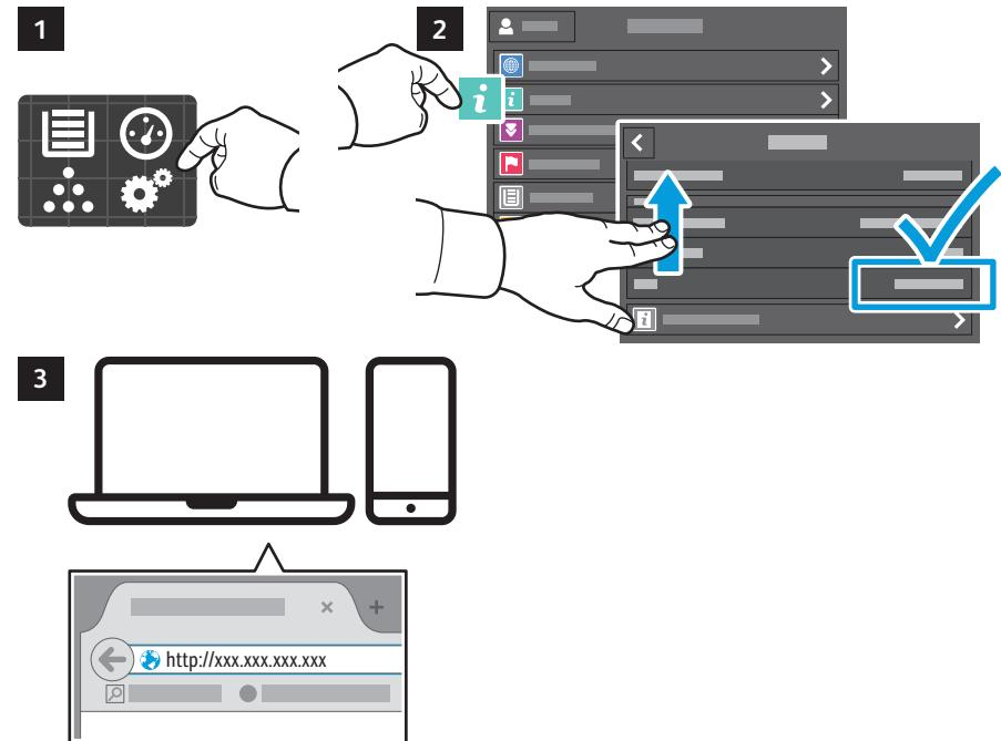
**EN** To connect, in a Web browser, type the printer IP address. The network IPv4 address is available on the control panel touch screen. Touch **Device** app > **About**, then scroll down.
