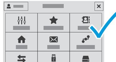
**EN** Scan To offers a variety of scan destinations to choose from and allows you to send to multiple destinations not accessible to single-purpose apps such as scanning to Email or USB. Touch **Scan To** then choose your first destination.
