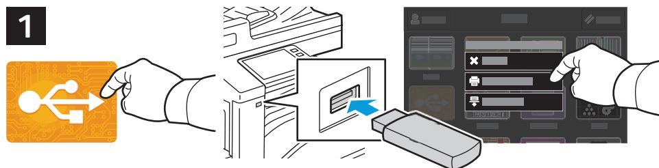
EN Scan to USB is a simple way to acquire a scan if you do not have prepared destinations or network access. Touch USB or insert your USB Flash Drive, then choose **Scan to USB**.
