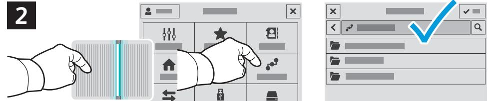
EN To scan to your prepared network location, touch Scan To... and choose Network. Select a subfolder as needed.
