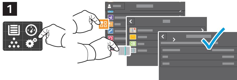
EN You can set up a scan-to folder on the network or online. To create a location, touch Device > Apps > Scan To... then choose Network or FTP. To scan to FTP, enter the FTP settings. To select a folder on the network or online, navigate to the desired location.
