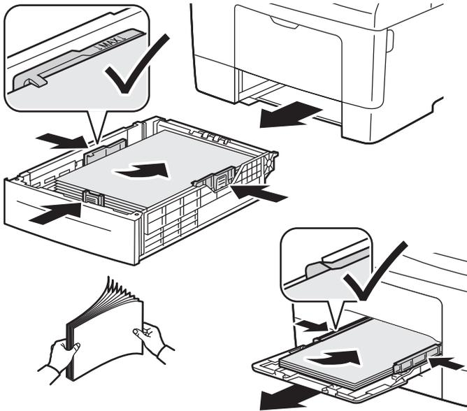
For best results, fan the edges of the paper. Adjust guides to fit the paper size. Do not load paper above the maximum fill line.
