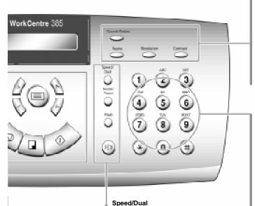
Use to dial calls and send fax documents by entering a 2-digit number. Also use to switch the LCD display between tasks while
