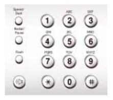
For example, to enter the letter O, press the 6 key (labeled MNO). Each time you press the 6 key, the display shows a different letter, first M, the N, and O, and finally 6.
