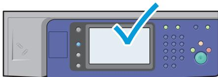
**EN** When a jam occurs, the control panel touch screen displays an animated graphic showing how to clear the jam.
