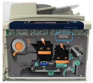
1. To access the serial number open the front door. The serial number is located on a label above the fuser module.
